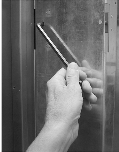
Figure 12. Expansion Bay Latches
